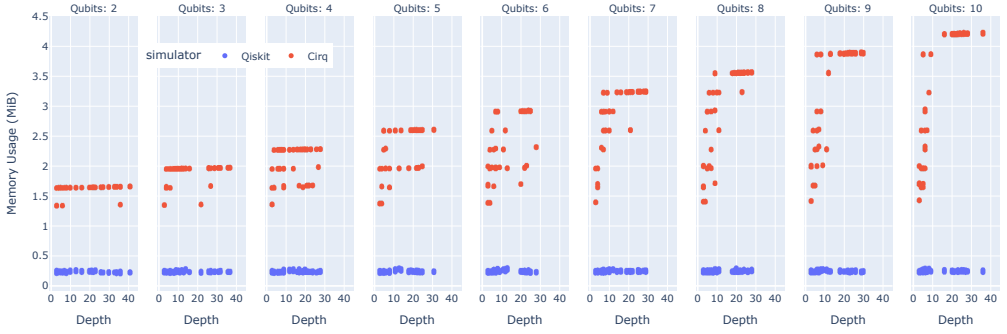
Fig. 9. Memory Usage in Qiskit and Cirq Simulators as a Function of Circuit Depth and Number of Qubits, with shaded regions highlighting different qubit ranges.
